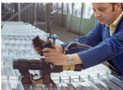
Partial shrinking of wings for Dornier Do 228
