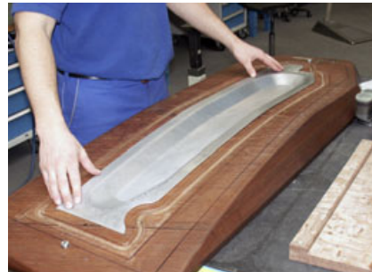
Correcting Job with Eckold forming machine KF460 of a lower covering part of of the floor section for the Airbus A380
