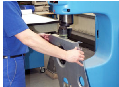
Correcting and adjusting of a pressed part of the fuselage section of an Airbus A340
